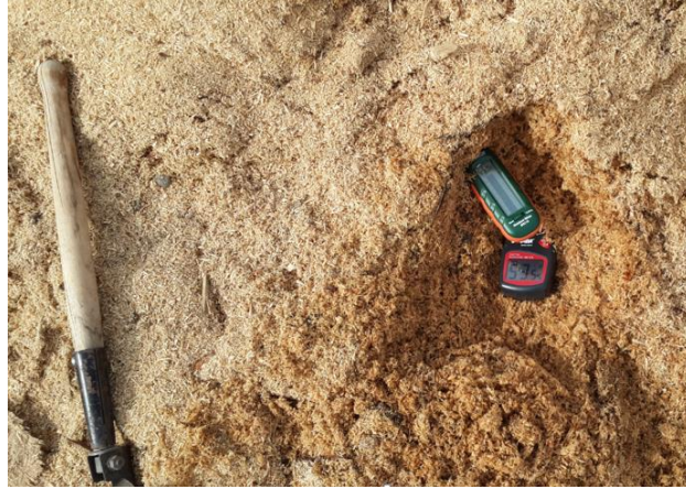
Pic 2. – Measuring the moisture content of the sawdust
